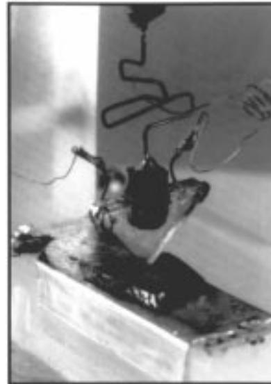
Fig. 2. The first transistor.
