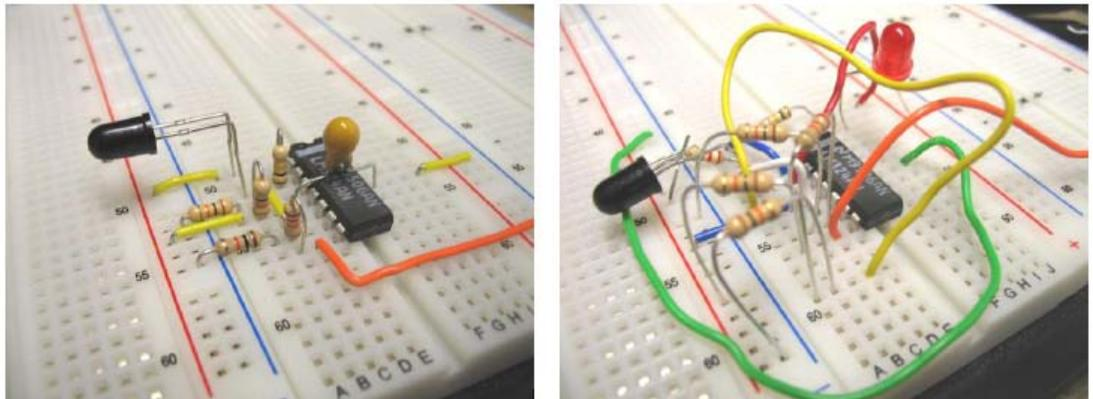
The proto-boards are fairly robust, however they are susceptible to damage from wires that are too large. Do not use hook-up wire larger than 24 gauge. This should not be a problem, since we are supplying hook-up wire kits. The other thing to watch for is component lead sizes. This will not be much of a problem during the labs, but you should be aware of these limitations since in later quarters you may use these boards to prototype your own circuits.
