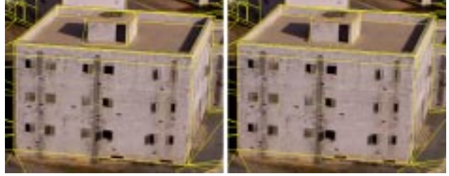
Figure 8. Refinement of object placement. (a) enlargement of Fig. 5b, showing errors in three-story building and structure on its roof; (b) alignment of model to image after refining object placements.
