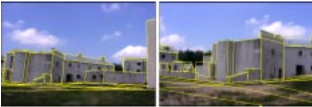
Figure 6. Alignment of untextured model to 100-frame ground-level video; (a) frame 25; (b) frame 90. See also Movie 7 in [19].
