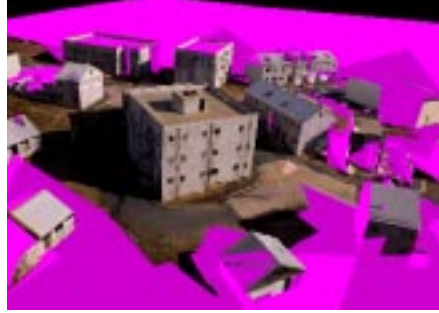
Figure 10. A view rendered from polyhedral model, with textures recovered from the entire aerial video sequence. Blank areas were never seen by the moving camera. See also Movie 8 in [19].
