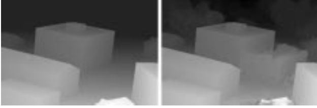
Figure 9. Refinement of surface shape. (a) Depth map implied by original model for the frame shown in Fig. 5d; (b) Estimation of residual parallax reveals previously unmodeled building and background trees.
